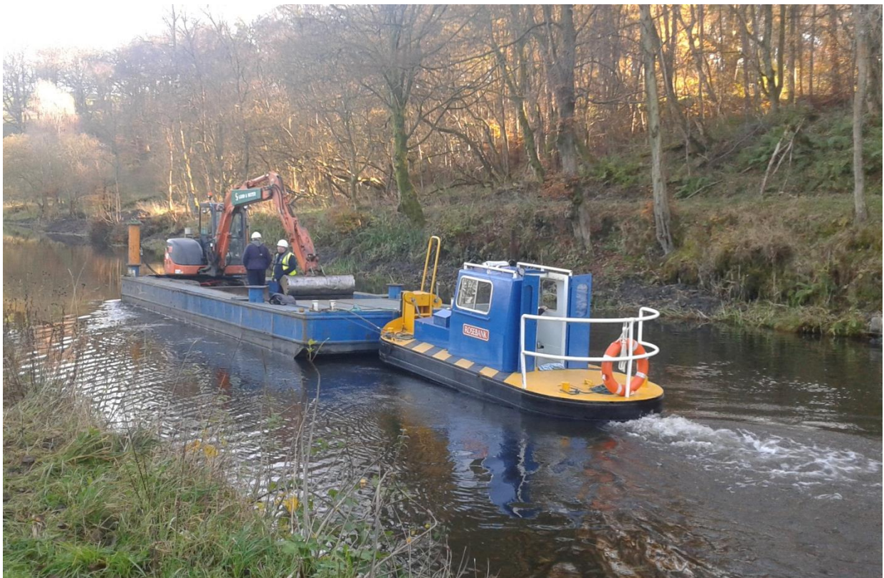
Above: tug pushing knockdown pontoon along Forth & Clyde Canal at Devil's Elbow
