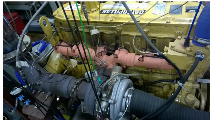
Caterpillar 3126B Tesbed : 6 cylindres 300CV
